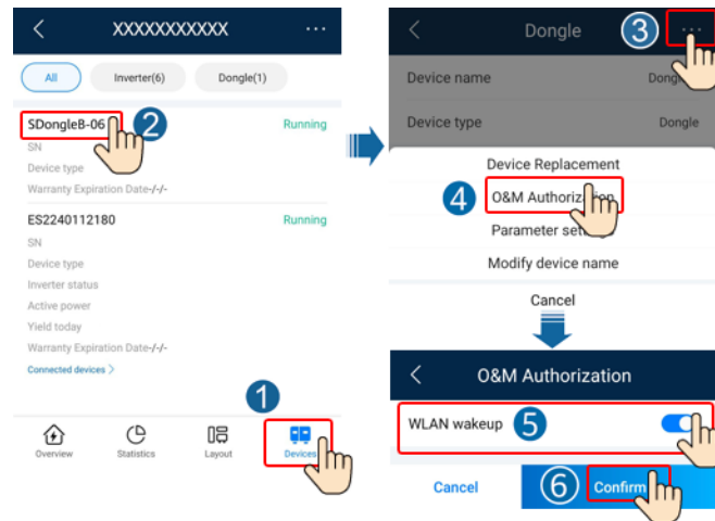
Figure 2-6 Enabling the Smart Dongle WLAN
