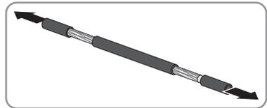
6. Attach each cable piece for shielding to a shield clamp. To do so, plug one end of each cable piece into the ring terminal lug of the shield clamp and crimp using a crimping tool.
