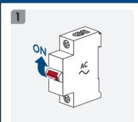
After installation and checking wiring turn on the circuit breaker.
