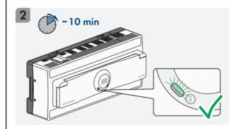
When power supply for the Data Manager M is available the device starts its boot sequence and searches for an initial update file.
