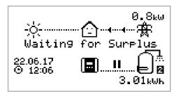
2. If there is more than one heater you may select which heater you wish to boost by pressing for to change heater. Press to start boost
