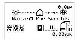
eddi is waiting for surplus power from the microgeneration system. The house in the centre is straight faced as grid electricity is being used by the house (0.8kW is this example).
