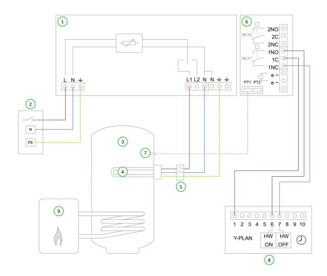
1eddi device5Isolator (20A double pole)2Mains supply (230V AC from B16 circuit breaker or<br/>13A fused spur)6Relay & Sensor Board (optional add-on for eddi)3Hot water cylinder7Temperature probe (type PT1000) (optional)4Water heating element (max. 3.7kW)8Y-Plan wiring centre9Auxiliary water heating boiler
